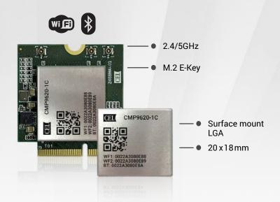
New wireless deployments demand more data throughput and more efficient network utilization. CEL designed the CMP9620 to deliver both, While offering out-of-the-box integration into NXP's I.MX8 ecosystem. Simultaneous Dual-Band operation, combined with concurrent Bluetooth and the latest Bluetooth features, deliver the connectivity demanded by Edge Gateways, HUBS and other High-Banwidth applications.
