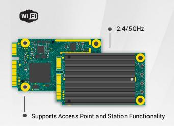
CEL's CMP964x was designed and built for ultra-high speed capability for enterprise and industrial Access Point applications. This dualband Wi-Fi 6 solution is capable of both Access Point and Station functionality, while supporting four simultaneous spatial streams of up to 160 MHz bandwidth. Delivering up to 4.8 Gbps theoretical throughput, the CMP964x supports PCI Express 3.0 dual-lane for the host interface.
